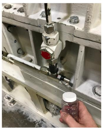
A proper sample represents the true condition of the equipment. It's taken while the equipment is running and it is taken from the same spot every time.
